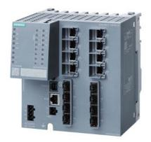
SCALANCE XM408-8C; managed modular IE switch; 8x 10/100/1000 Mbit/s RJ45; 8x 100/1000 Mbit/s SFP; contains 8 combo ports; in total 8 ports can be used; expandable to 24 ports electrical or optical; assembly: DIN rail/S7 mounting rail, PROFINET IO device; redundancy functions; office features (RSTP, VLAN, IGMP,..); C-PLUG in scope of supply; layer 3 integrated.
