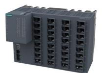
SCALANCE XC332 managed Layer 2 IE switch, 32x 10/100/1000 Mbit/s RJ45, LED diagnostics, error-signaling contact with select/set pushbutton, PROFINET IO device, network management, redundancy functions, office features (RSTP, VLAN, IGMP,..) CLP included in scope of supply assembly: DIN rail/S7 mounting rail .
