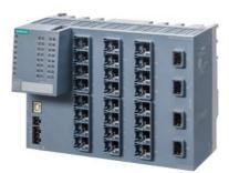
SCALANCE XC324-4 managed layer 2 IE switch, 24x 10/100/1000 Mbit/s RJ45, 4x 1/10 Gbit/s SFP+ port, LED diagnostics,error signaling contact with select/set pushbutton, PROFINET IO device, network management, redundancy functions, office features (RSTP, VLAN, IGMP,..) CLP included in scope of supply assembly: DIN rail/S7 mounting rail .
