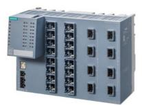
SCALANCE XCM324 managed layer 2 IE switch, 16x 10/100/1000 Mbit/s RJ45, 8x 1/10 Gbit/s SFP+ port, LED diagnostics,error signaling contact with select/set pushbutton, PROFINET IO device, network management, redundancy functions, office features (RSTP, VLAN, IGMP,..) CLP included in scope of supply assembly: DIN rail/S7 mounting rail .
