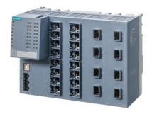
SCALANCE XC316-8 managed layer 2 IE switch, 16x 10/100/1000 Mbit/s RJ45, 8x 1/10 Gbit/s SFP+ port, LED diagnostics, error signaling contact with select/set pushbutton, PROFINET IO device, network management, redundancy functions, office features (RSTP, VLAN, IGMP,...) CLP included in scope of supply assembly: DIN rail/S7 mounting rail.
