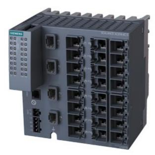
SCALANCE XC224-4C G manageable layer 2 IE Switch; Full Gigabit; 20x 10/100/1000 Mbps RJ45 ports; 4x 1000 Mbps combo ports (either 1000 Mbps s SFPs or 10/100/1000 Mbps RJ45 ports can be used); 1x console port; Diagnostic LED; redundant power supply; Temp. range -40 °C to +70 °C; Mounting: Standard mounting rail/S7 mounting rail/wall; redundancy functions; office features (RSTP, VLAN ,...); PROFINET IO Device; Ethernet/IP conformity; C-PLUG shaft;
