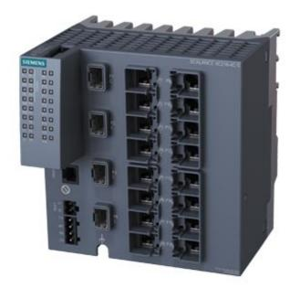
SCALANCE XC216-4C G manageable layer 2 IE Switch; Full Gigabit; 12x 10/100/1000 Mbps RJ45 ports; 4x 1000 Mbps combo ports (either 1000 Mbps s SFPs or 10/100/1000 Mbps RJ45 ports can be used); 1x console port; Diagnostic LED; redundant power supply; Temp. range -40 °C to +70 °C; Mounting: Standard mounting rail/S7 mounting rail/wall; redundancy functions; office features (RSTP, VLAN ,...); PROFINET IO Device; Ethernet/IP conformity; C-PLUG shaft;
