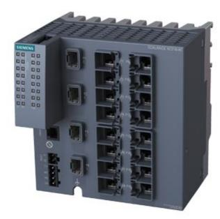
SCALANCE XC216-4C Manageable Layer 2 IE Switch; 12x 10/100 Mbit/s RJ45 ports; 4x 1000 Mbit/s combo ports (either 1000 Mbit/s SFPs or 10/100/1000 Mbit/s RJ45 ports can be used); 1x console port; diagnostics LED; Redundant power supply; Temp. range -40 °C to +70 °C Mounting: Standard mounting rail/S7 mounting rail/wall; Redundancy functions; Office features (RSTP, VLAN, etc.); PROFINET IO device; Ethernet/IP-compliant; C-PLUG slot;
