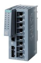
SCALANCE XC208G manageable Layer 2 IE switch; IEC 62443-4-2 certified; 8x 10/100/1000 Mbps; RJ45 ports; 1x console port; diagnostics LED; redundant power supply; temperature range -40 °C to +70 °C; assembly: DIN rail/S7 mounting rail/wall redundancy functions; office features (RSTP, VLAN,...); PROFINET IO device; Ethernet/IP-compliant; C-PLUG slot; IEEE 1588v2 PTP
