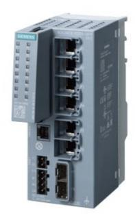
SCALANCE XC206-2SFP EEC Manageable layer 2 IE switch 6x 10/100 Mbit/s RJ45 ports; 2x 100/1000 Mbit/s SFP; 1x console port; Diagnostics LED; Redundant power supply; with painted printed circuit boards; NAMUR NE21-compliant; Temp. range -40 °C to +70 °C Mounting: Standard mounting rail/S7 mounting rail/wall; Redundancy functions; Office features (RSTP, VLAN,...); PROFINET IO device; Ethernet/IP-compliant; C-PLUG slot;
