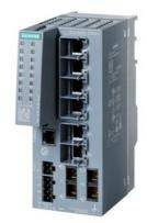
SCALANCE XC206-2 manageable Layer 2 IE switch; IEC 62443-4-2 certified; 6x 10/100 Mbit/s RJ45 ports; 2x 100 Mbit/s SC-ports, 1x console port; diagnostics LED; redundant power supply; temperature range -40 °C to +70 °C; assembly: DIN rail/S7 mounting rail/wall; redundancy functions; office features (RSTP, VLAN,...); PROFINET IO device Ethernet/IP-compliant C-PLUG slot.
