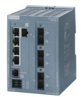
SCALANCE XB205-3 managed Layer 2 IE Switch 5x IEC 62443-4-2 certified; 10/100 Mbit/s RJ45 ports 3x MM FO SC-port 1x console port, diagnostics LED redundant power supply; IEC 62443-4-2 certified; temperature range 0 °C to +60 °C; DIN-rail mounting; default EtherNet/IP.
