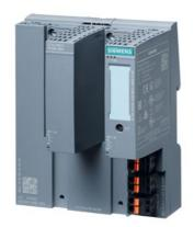
SCALANCE XF204-2BA managed IE switch, 4 x 10/100 Mbit/s, IEC 62443-4-2 certified; 2 x BusAdapter interface, error signaling contact, set pushbutton, redundant 24 V DC power supply, PROFINET device, extended temperature range -40 °C...+70 °C, conformal coating, with electr. manual on DVD, C-PLUG optional, supplied without BusAdapter
