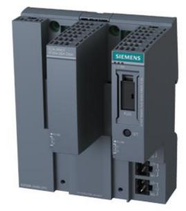
SCALANCE XF204 DNA managed IE Y-Switch, 2 Bus adapter BA 2xRJ45 HA,pre- assembled 6DL1193-6AR00-0AA0 4 x 10/100Mbit/s, 2 x Bus adapter interface, Error signaling contact with set button, redundant 24V DC power supply, PROFINET-Device, extended temperature range -40°C to +70°C, Conformal Coating, with electr.. manual on DVD, C-PLUG optional, Delivery with bus adapter
