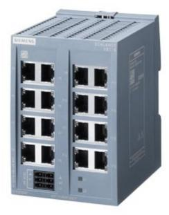
SCALANCE XB116 unmanaged IE switch, 16x 10/100 Mbit/s RJ45 ports; for setting up small star and line topologies; LED diagnostics, IP20, Redundant power supply, 24 V AC/DC Manual available as a download
