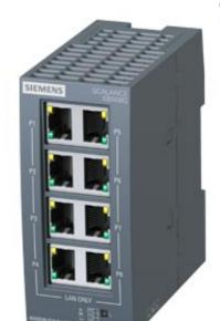
SCALANCE XB008G unmanaged Industrial Ethernet Switch for 10/100/1000 Mbit/s; for setting up small star and line topologies; LED diagnostics, IP20, 24 V DC power supply, with 8x 10/100/1000 Mbit/s RJ45 ports electrical Manual available as a download
