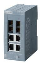
SCALANCE XB004-2 unmanaged Industrial Ethernet Switch for 10/100 Mbit/s; for setting up small star and line topologies; LED diagnostics, IP20, 24 V DC power supply, with 4x 10/100 Mbit/s twisted pair ports with RJ45 sockets; 2x 100 Mbit/s multimode glass fiber-optic cable port with SC socket; manual available as a download .
