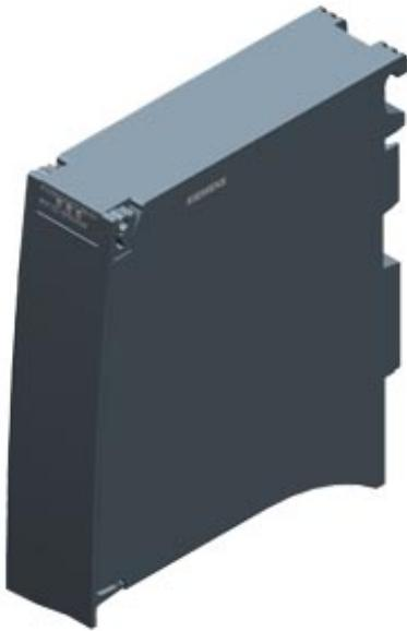
SIMATIC S7-1500 digital input/output module, DI 32x24VDC BA SNK / SRC, 32 channels in groups of 16, input delay typ. 3.2 ms input type 3 (IEC 61131), sinking/sourcing input, DQ 32XDC 24V/0.3A SNK BA; 32 channels in groups of 16; 2 A per group at 60 °C; sourcing output; 35 mm wide; cables and terminal blocks to be ordered separately as accessories
