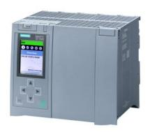
SIMATIC S7-1500T, CPU 1518T-4 PN/DP, central processing unit with 9 MB work memory for program and 60 MB for data, 1st interface: PROFINET IRT with 2-port switch, 2nd interface: PROFINET RT, 3rd interface: PROFINET basic services, 4th interface: PROFIBUS, 1 ns bit performance, SIMATIC memory card required
