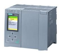
SIMATIC S7-1500TF, CPU 1517TF-3 PN/DP, Central processing unit with work memory 3 MB for program and 8 MB for data, 1st interface: PROFINET IRT with 2-port switch, 2nd interface, Ethernet, 3rd interface, PROFIBUS, 2 ns bit performance, SIMATIC Memory Card required
