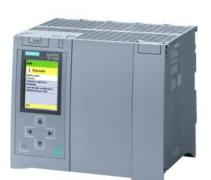
SIMATIC S7-1500TF, CPU 1516TF-3 PN/DP, Central processing unit with 1.5 MB RAM for program and 5 MB for data, 1st interface: PROFINET IRT with 2-port switch, 2nd interface, Ethernet, 3rd interface, PROFIBUS, 10 ns bit performance, SIMATIC Memory Card required
