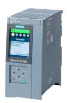
SIMATIC S7-1500, CPU 1516-3 PN/DP, central processing unit with 2 MB work memory for program and 7.5 MB for data 1st interface: PROFINET IRT with 2-port switch, 2nd interface: PROFINET RT, 3rd interface: PROFIBUS, 6 ns bit performance, SIMATIC Memory Card required \*\*\* approvals and certificates according to entry 109816732 at support.industry.siemens.com to be considered! \*\*\*
