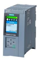
SIMATIC S7-1500T, CPU 1515TF-2 PN, central processing unit with 1.5 MB work memory for program and 4.5 MB for data, 1st interface: PROFINET IRT with 2-port switch, 2nd interface: PROFINET RT, 6 ns bit performance, SIMATIC Memory Card required \* \*\*\* approvals and certificates according to entry 109816881 at support.industry.siemens.com to be observed! \*\*\*\*
