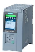
SIMATIC S7-1500, CPU 1515-2 PN, central processing unit with work memory 1 MB for program and 4.5 MB for data, 1st interface: PROFINET IRT with 2-port switch, 2nd interface: PROFINET RT, 6 ns bit performance, SIMATIC Memory Card required \*\*\* approvals and certificates according to entry 109816732 at support.industry.siemens.com to be considered! \*\*\*
