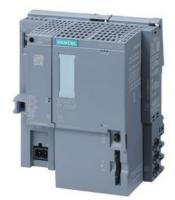
SIMATIC DP, CPU 1514SP T-2 PN for ET 200SP, central processing unit with work memory 900 KB for program and 3.5 MB for data, 1st interface: PROFINET IRT with 2-port switch, 2nd interface: PROFINET RT 6 ns bit performance, SIMATIC Memory Card required, BusAdapter required for 1st interface \*\*\*\* approvals and certificate entry 109817813 at support.industry.siemens.com \*\*\*\*
