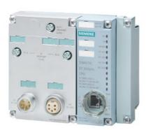
SIMATIC DP, CPU 1513pro-2 PN for ET 200pro, central processing unit with 300 KB work memory for program and 1.5 MB for data, 1st interface: PROFINET IRT with 3-port switch, 2nd interface: PROFINET RT, 40 ns bit performance, Degree of protection: IP65/67, SIMATIC Memory Card required connection module required
