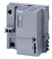
SIMATIC DP, CPU 1510SP F-1 PN for ET 200SP, central processing unit with work memory 300 KB for program and 1 MB for data, 1st interface: PROFINET IRT with 3-port switch, 25 ns bit performance, SIMATIC Memory Card required, BusAdapter required for port 1 and 2 \* \*\*\* approvals and certificates according to entry 109817615 at support.industry.siemens.com to be observed! \*\*\*\*
