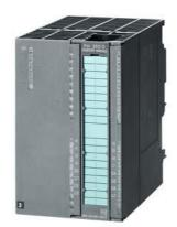
SIMATIC S7-300, Counter module FM 350-2, 8 channels, 20 kHz, 24 V encoder for  $counting, frequency\ measurement,\ speed\ measurement,\ period\ duration$ measurement, dosing incl. configuration package and electronic documentation on
