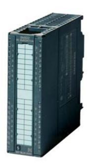
SIMATIC S7-300, DIGITAL OUTPUT SM 322, OPTICALLY ISOLATED, 8 DO (RELAY), 1 X 40 PIN, 24V DC, 5A OR 230V AC, 5A, CONNECTOR W.SPRING TERMINAL CAN BE USED FROM 6ES7392-1BM01-0AA0
