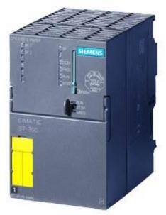
\*\*\* SPARE PART\*\*\* SIMATIC S7-300 CPU317F-2 PN/DP, CENTRAL PROCESSING UNIT WITH 1024 KBYTE WORKING MEMORY, 1. INTERFACE MPI/DP 12MBIT/S, 2. INTERFACE ETHERNET PROFINET, MICRO MEMORY CARD NECESSARY FOR USE WITH SOFTWARE OPTION S7 DISTRIBUTED SAFETY V5.4 OR HIGHER
