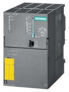
\*\*\*Spare part\*\*\* SIMATIC S7-300 CPU315F-2 PN/DP, Central processing unit with 256 KB work memory, 1st interface MPI/DP 12 Mbit/s, 2nd interface Ethernet PROFINET, Micro Memory Card required Can be used with software package S7 Distributed Safety from V5.4
