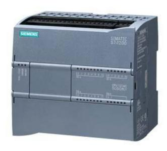
SIMATIC S7-1200, CPU 1214C, COMPACT CPU, DC/DC/RELAY, ONBOARD I/O: 14 DI 24V DC; 10 DO RELAY 2A; 2 AI 0 - 10V DC,
