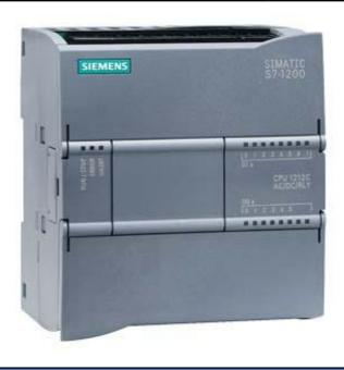
SIMATIC S7-1200, CPU 1212C, COMPACT CPU, AC/DC/RLY, ONBOARD I/O: 8 DI 24V DC; 6 DO RELAY 2A; 2 AI 0 - 10V DC,
