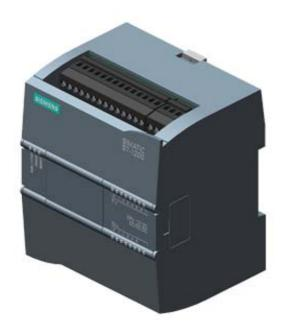
SIMATIC S7-1200, CPU 1212C, COMPACT CPU, DC/DC/DC, ONBOARD I/O: 8 DI 24V DC; 6 DO 24 V DC; 2 AI 0 - 10V DC,
