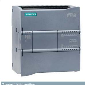
\*\*\* SPARE PART\*\*\* SIMATIC S7-1200, CPU 1212C, COMPACT CPU, DC/DC/DC, ONBOARD I/O: 8 DI 24V DC; 6 DO 24 V DC; 2 AI 0 - 10V DC, POWER SUPPLY: DC 20.4 - 28.8 V DC, PROGRAM/DATA MEMORY: 25 KB
