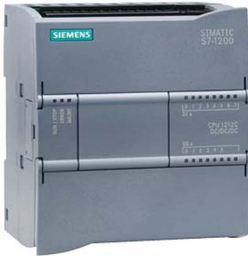
\*\*\* SPARE PART\*\*\* SIMATIC S7-1200, CPU 1212C, COMPACT CPU, DC/DC/DC, ONBOARD I/O: 8 DI 24V DC; 6 DO 24 V DC; 2 AI 0 - 10V DC, POWER SUPPLY: DC 20.4 - 28.8 V DC, PROGRAM/DATA MEMORY: 25 KB
