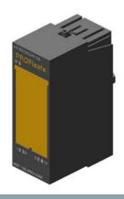
\*\*\* Spare part \*\*\* SIMATIC DP, Electronics module for ET 200S, 4 F-DO PROFIsafe, 24 V DC/2 A, 30 mm overall width, up to PL E (ISO 13849), up to SIL 3 (IEC 61508), can also be used in PROFINET configuration with IM 151-3 HF
