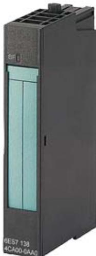
SIMATIC DP, ELECTRONIC MODULE FOR ET 200S, 2 AO I 15 MM WIDE, +/-20 MA; 13 BIT + SIGN, 4 .. 20 MA; 13 BIT CYCLE TIME < 1 MS WITH LED SF (GROUP FAULT)
