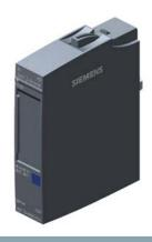
SIMATIC ET 200SP, Analog input module, Al 2x U/I 2-.4-wire High Speed, suitable for BU type A0, A1, Color code CC00, channel diagnostics, 16 bit, +/-0.3%
