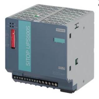
SITOP UPS500S BASIC UNIT 5 KWS SITOP UPS500S service-free uninterruptible power supply with USBinterface basic unit 5 kWs input: 24 V DC output: 24 V/15 A DC degree of protection IP20
