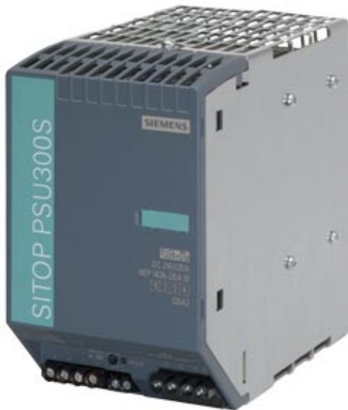
SITOP PSU300S 20 A STABILIZED POWER SUPPLY INPUT: 400-500 V 3 AC OUTPUT: 24 V DC/20 A
