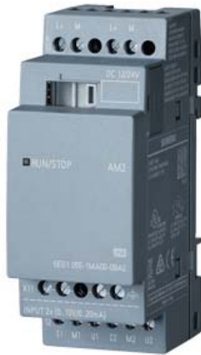
LOGO! AM2 EXPANSION MODULE, PU: DC 12/24V, 2 AI, 0 - 10V OR 0/4 - 20mA FOR LOGO! 8
