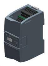
SIPLUS S7-1200 SM 1234 4AI/2AQ rail based on 6ES7234-4HE32-0XB0 with conformal coating, -25...+60 °C, OT1 with ST1/2 (+70 °C für 10 minutes), SM 1234, 4 AI/2 AQ, +/-10 V, 14-bit resolution or 0 (4)-20 mA, 13-bit resolution
