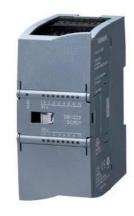
SIPLUS S7-1200 SB 1223 2DI/2DQ T1 rail based on 6ES7223-0BD30-0XB0 with conformal coating, -25...+55 °C, OT1 with ST1/2 (+70 °C für 10 minutes), digital input/output 2 DI 24 V DC/2 DQ 24 V DC
