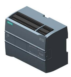
SIPLUS S7-1200 CPU 1215C DC/DC/DC -40...+70°C with conformal coating based on 6ES7215-1AG40-0XB0 . compact CPU, DC/DC/DC, 2 PROFINET ports, onboard I/O: 14 DI 24 V DC 10 DO 24 V DC 0.5 A 2 AI 0-10 V DC, 2 AO 0-20 mA DC, Power supply: DC 20.4-28.8V DC, Program/data memory 125 KB
