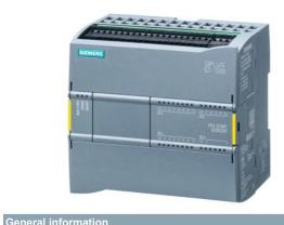
SIPLUS S7-1200 CPU 1214FC DC/DC/relay based on 6ES7214-1HF40-0XB0 with conformal coating, -25...+55 °C, compact CPU, DC/DC/relay, onboard I/O: 14 DI 24 V DC; 10 DQ relay 2 A; 2 AI 0-10 V DC, power supply: DC 20.4-28.8 V DC, program/data memory 125 KB
