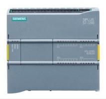
SIPLUS S7-1200 CPU 1214FC DC/DC/DC based on 6ES7214-1AF40-0XB0 with conformal coating, -25...+55 °C, compact CPU, DC/DC/DC, onboard I/O: 14 DI 24 V DC; 10 DQ 24 V DC; 2 AI 0-10 V DC, power supply: DC 20.4-28.8 V DC, program/data memory 125 KB
