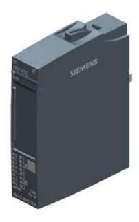
SIPLUS ET 200SP, digital input module, DI 16X DC 24V standard, - 40...+70°C with conformal coating based on 6ES7131-6BH01-0BA0 . type 3 (IEC 61131), sink input, (PNP, P-reading), Packing unit: 1 Piece, passend für BU-Typ A0, Farbcode CC00, Modul-Diagnose input delay time 0,05..20ms, diagnostics wire break, diagnostics supply voltage
