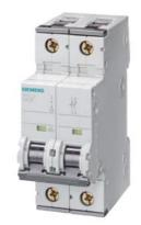
Miniature circuit breaker 400 V 15kA, 2-pole, C, 2A, D=70 mm
