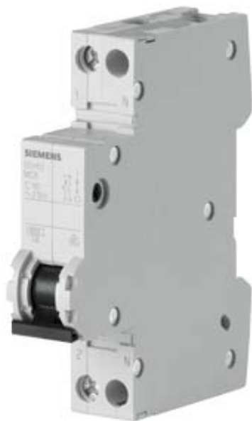
CIRCUIT-BREAKER 230V 6KA, 1+N-POLE/1MW, C 10A
