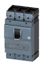
circuit breaker 3VA1 IEC frame 630 breaking capacity class C Icu=110kA @ 415 V 3-pole, starter protection TM120M, AM, In=500A without overload protection short-circuit protection Ii=8...16 x In nut keeper kit
